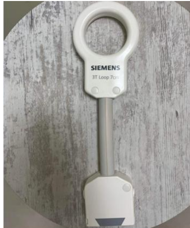
Fig. 4.1. Specialized eye socket coil
